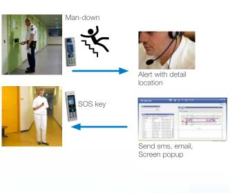
ensures that when the handset or Messenger SOS button is used, or when the handset shows a man-down indication, a central alert is given including escalation by means of a variety of media, such as sms, email or by voice conversation. This is facilitated by Ekahau Vision and can be further enhanced with a dedicated messaging system to escalate to other staff members using their DECT handset messaging.
